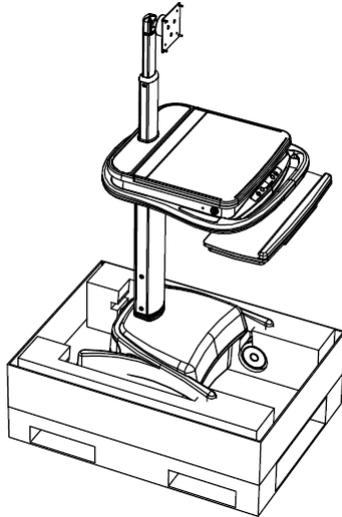
**4** Remove cardboard walls and plastic bag. NOTE: This step requires two people. Lift cart (with foam castor braces still attached) out of the cardboard base.
